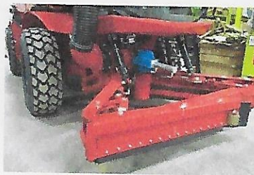
FOLDING BLADE Wings in and out operated by joystick
